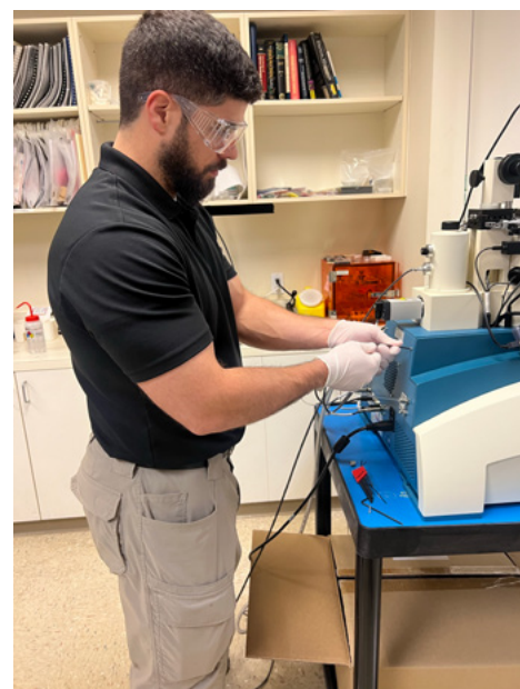
Senior Engineer Dan Foley practices loading a sample into the PECS ion mill.
